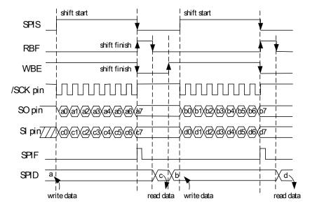
Fig. 17. Transmit/Receive Mode (8-bit, 1 word)
